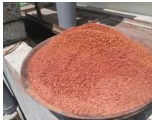
Figure(3) 2.36mm retained grain size
