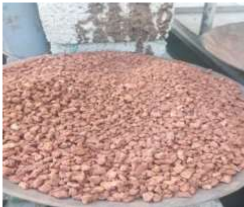
Figure(2) 4.75mm retained grain size
